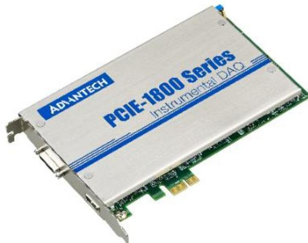
The card offers 115 dB dynamic range, with input voltages being anywhere from +/- 0.2 to 10 V. It also has full auto-calibration and a built-in anti-aliasing filter, ensuring that the conversion of incoming signals is as free of artifacts and errors as possible.
